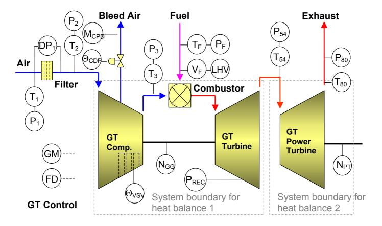
LM 2500 process measuring positions (these signals are easily imported to COMPASS<sup>™</sup> and used for judging the performance condition of the gas turbine).
