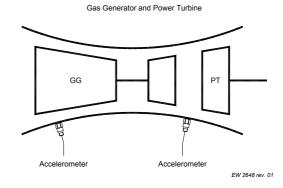
Vibration sensor instrumentation for a General Electric **LM 2500** gas turbine (2 shafts: gas generator and power turbine).
