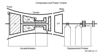
Vibration sensor instrumentation for a **Rolls-Royce RB211** gas turbine, comprising of a 2 shafts gas generator and a power turbine.
