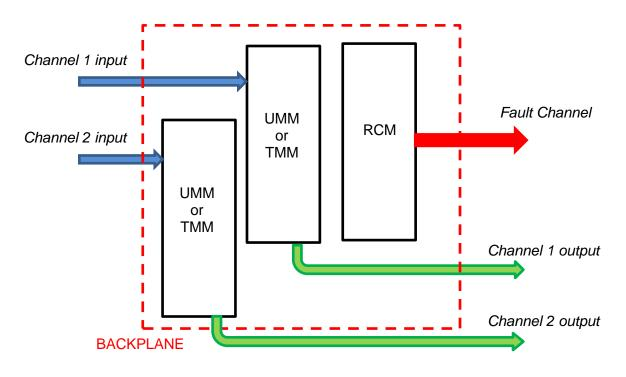
This architecture is characterized by the use of two different cards to acquire two independent signals coming from two sensors installed so as to measure the same process variable, in order to realize a redundancy of the measurement. The effectiveness of the redundancy in terms of measurement is under the end-user responsibility such as the correct selection of all devices not included in the MPS-VC8000.
