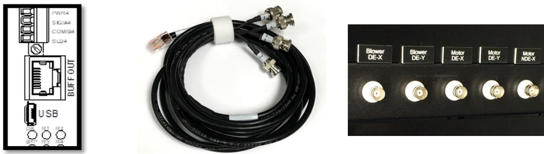
Figure 53: Buffered output connectors
