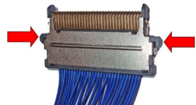
Figure 94: Display Connector Retention Locks
